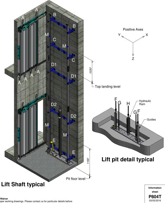
The data sheet is for guidance only & must not be used for proper working drawings. Please contact us for particular details before proceeding. Owing to our policy of continual improvement, we reserve the right to alter specifications & dimensions without prior notice.
